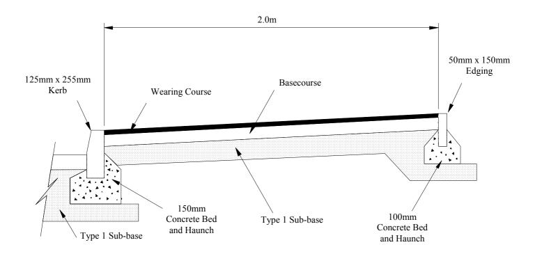
Figure 3.1 : Typical Pedestrian-only Footway Cross-section
