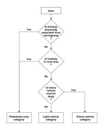
Pedestrian-only : Light-vehicle : Heavy-vehicle : Footways designed for pedestrian use only. Footways which will support overrun by light vehicles Footways which will support overrun by heavy vehicles.
